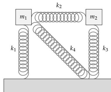
Figure 3.4: Take the truss in Figure 3.2 (with  $L_1 = L_2 = L_3$ ) and add a diagonal brace that meets the second spring at an angle of  $\pi/4$ .
