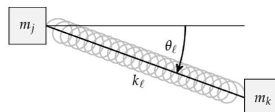
Figure 3.3: A spring's angle is measured clockwise, from the vertical.
