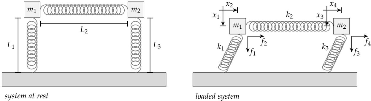
Figure 3.2: A tipsy table. Three springs with rest lengths  $L_j$  and spring constants  $k_j$  are connected via two masses,  $m_1$  and  $m_2$ . Forces vertical ( $f_1$  and  $f_3$ ) and horizontal ( $f_2$  and  $f_4$ ) are applied to each mass, causing vertical ( $x_1$  and  $x_3$ ) and horizontal ( $x_2$  and  $x_4$ ) displacements of each mass.
