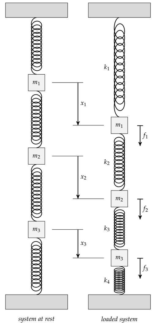
Figure 3.1: Four springs stacked vertically, separated by three masses and fixed at the top and bottom. The figure on the left shows the network with no load applied. When forces  $f_1$ ,  $f_2$ , and  $f_3$  are applied to the masses  $m_1$ ,  $m_2$ , and  $m_3$ , the springs deform, as sketched in the schematic on the right. These forces cause the  $j$ th mass to drop by  $x_j$  units, as controlled by the spring constants  $k_1, \dots, k_4$ .
