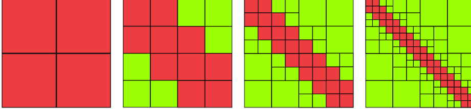
FIGURE 5. Construction of the block tree partition at level 1,2,3,4 of call of the build_block_tree function. The green blocks are admissible : at the end, only blocks of size < C_{leaf} are not admissible (pink). This matrix corresponds to a discretized 1D Laplace operator.
