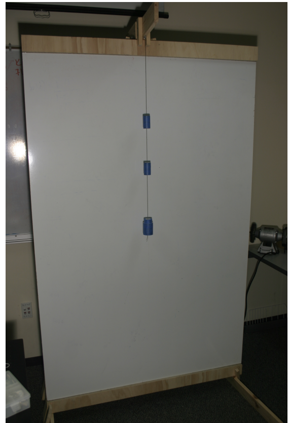
Figure 8.4: Experimental set-up: three masses are suspended on a flexible cable.
