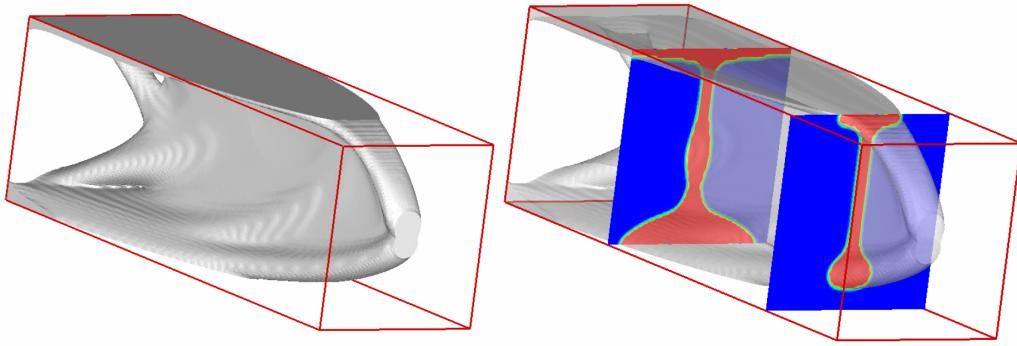
**FIGURE 4.** A cantilever beam solved in the FGM domain using the preconditioned, recycling MINRES solver and the CAMD approach; mesh size:  $210 \times 70 \times 70$  B8/B8 elements; total number of unknowns: approximately 1.6 million. Left: final design of FGM beam. Right: two cross-sections from the final design.
