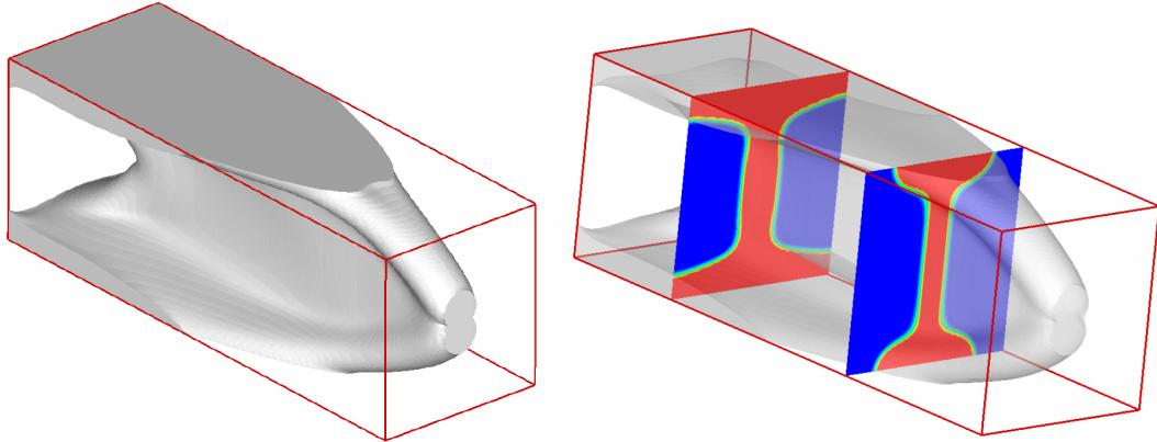
**FIGURE 3.** A cantilever beam design solved using the preconditioned, recycling MINRES solver and the CAMD approach; mesh size:  $210 \times 70 \times 70$  B8/B8 elements; total number of unknowns: approximately 1.6 million. Left: final design of an homogeneous material. Right: Two cross-sections from the final design.
