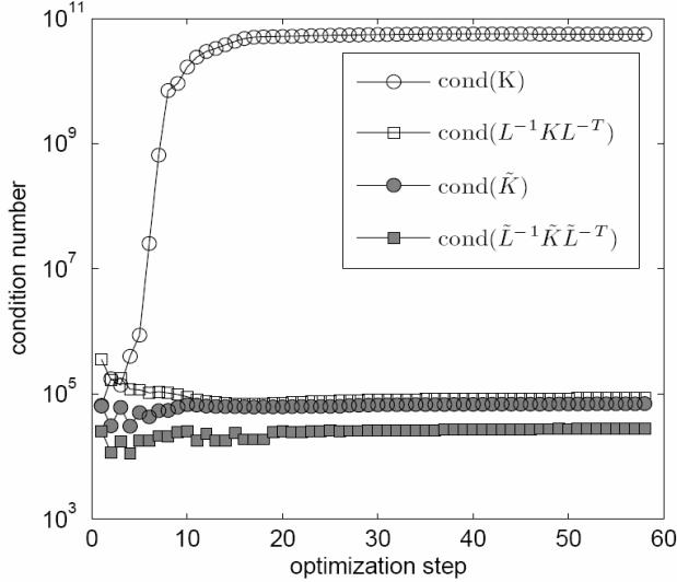
**FIGURE 1.** Condition numbers for (1) the original stiffness matrices,  $\mathbf{K}$ , (2) their incomplete Cholesky preconditioned forms,  $\mathbf{L}^{-1}\mathbf{K}\mathbf{L}^{-T}$ , (3) the diagonally scaled stiffness matrices,  $\tilde{\mathbf{K}}$ , and (4) their incomplete Cholesky preconditioned forms,  $\tilde{\mathbf{L}}^{-1}\tilde{\mathbf{K}}\tilde{\mathbf{L}}^{-T}$ .
